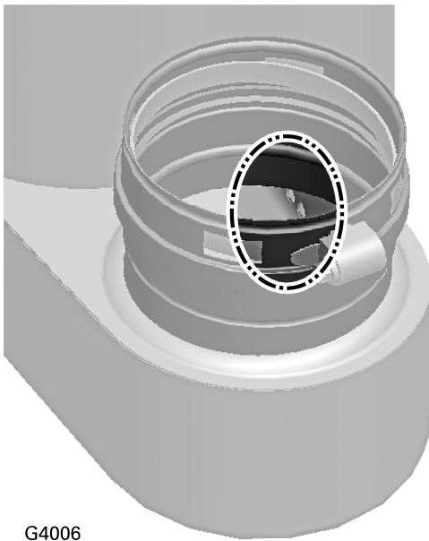
Figure 79 Recuperator flueway drain holes
