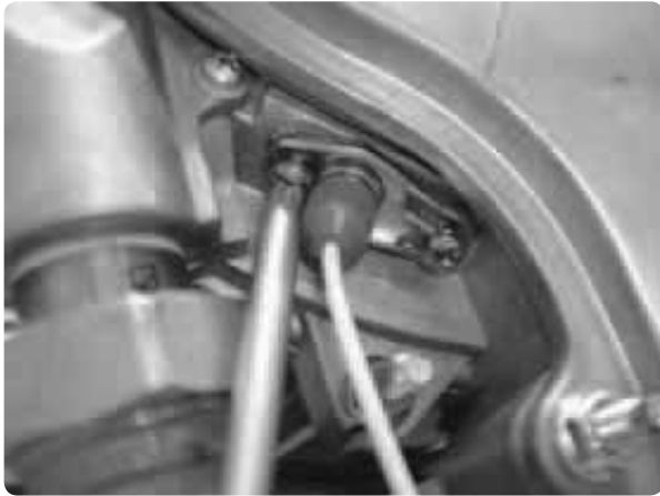
Figure 142 Removal of Ignition electrode
