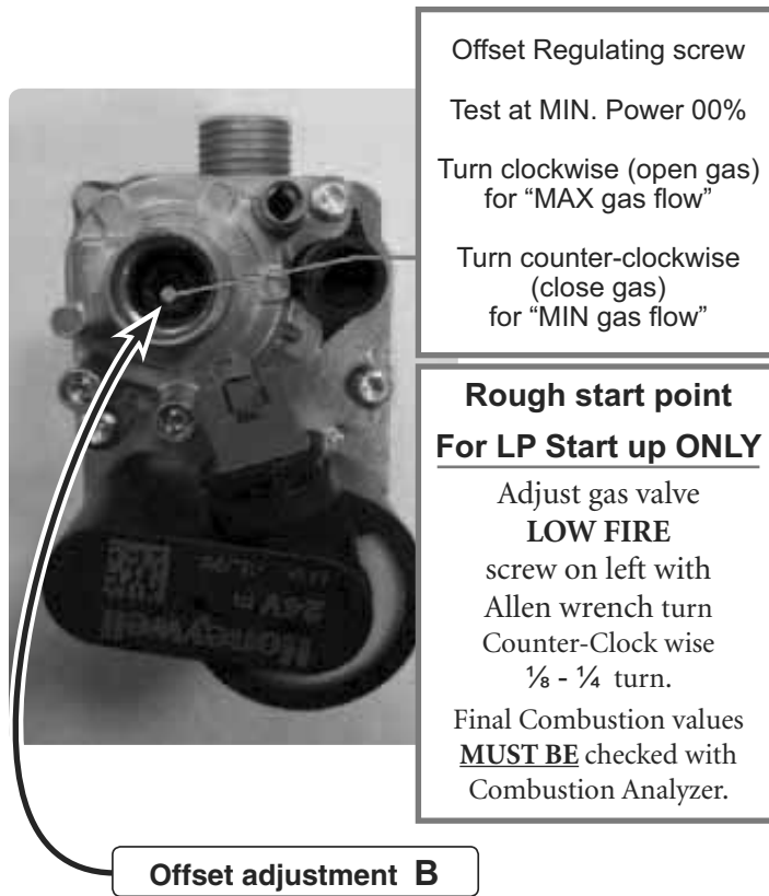
Figure 109 Offset adjustment screw — (ONLY for use by a qualified technician, using calibrated combustion test instruments).
