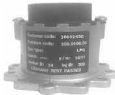
Figure 9 Liquefied Petroleum (propane) gas venturi label information
