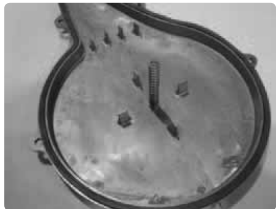
Figure 145 Heat exchanger cover plate removed
