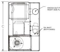
LOCATOR KNOCK-OUTS FOR RETURN AIR ON BOTH SIDES SIDE VIEW
