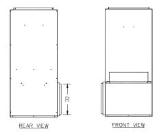
Note 1: Attach an external filter rack after cutting opening in side for return air duct connection. Either side can be used.
