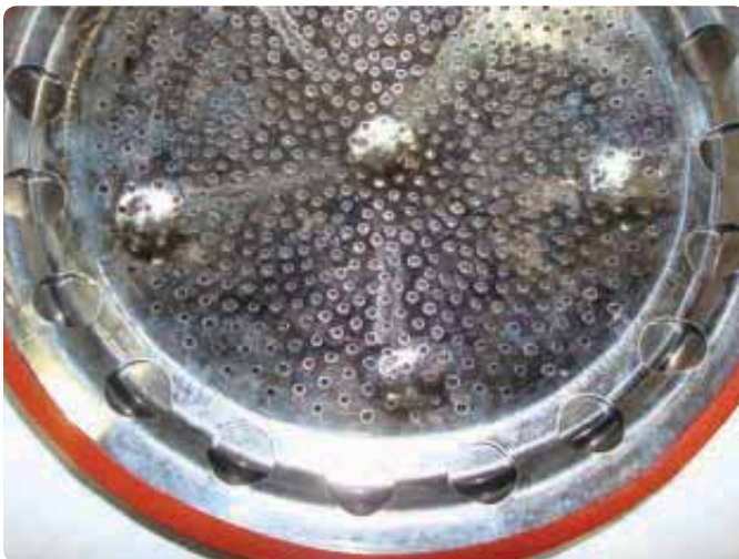
Figure 143 Inspecting interior and cleaning the burner
