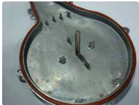
Figure 141 Heat exchanger cover plate removed
