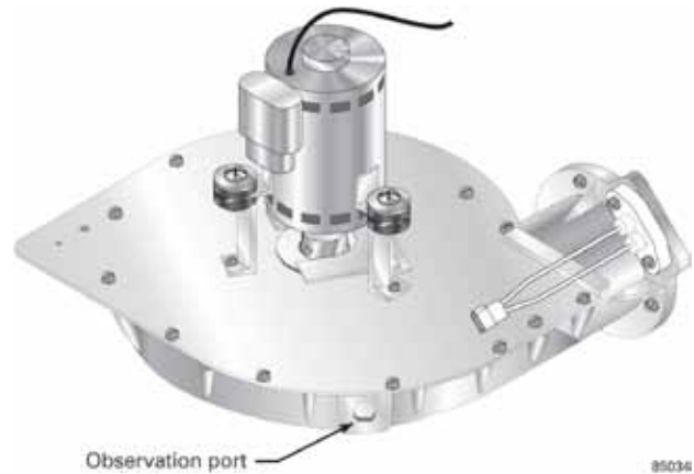
Figure 68 Check for igniter glow by looking into observation port on front of blower housing
