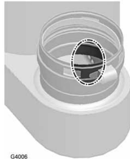
Figure 80 Recuperator flueway drain holes
